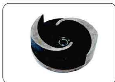
E: Unshrouded impeller, non clog, double channel design for good balance and smooth running. For high head with big flow.
